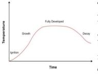
The Traditional Fire Development Curve shows the time history of a fuel-limited fire. In other words, the fire growth is not limited by a lack of oxygen. As more fuel becomes involved in the fire, the energy level continues to increase until all of the fuel available is burning (fully developed). Then as the fuel is burned away, the energy
