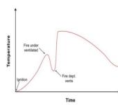
The Fire Behavior in a Structure Curve demonstrates the time history of a ventilation limited fire. In this case, the fire starts in a structure which has the doors and windows closed. Early in the fire growth stage there is adequate oxygen to mix with the heated gases, which results in flaming combustion. As the oxygen level within the
