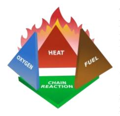
This is commonly called the fire tetrahedron. Fire cannot exist without all of these elements in place, and in the right proportions. For example, a flammable liquid will start burning only if the fuel and oxygen are in the right proportions. Some fueloxygen mixes may require a catalyst: a substance that is not consumed, when added, in any chemical reaction during combustion, and enables the reactants to combust more readily.
